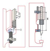
THE UPPER BEAM IS GUIDED BY 4 PAIRS OF BEARINGS THAT SLIDE, ALONG THE MACHINE'S SIDES, ON TRACKS OF HARDENED AND RECTIFIED STEEL. THE ALIGNMENT AND CENTERING OF THE BEAMS IS GUARANTEED BY THE GREAT DISTANCE BETWEEN THE UPPER AND LOWER BEARINGS (E). BOTH THE OPTICAL SCALES ARE CONNECTED TO THE CNC, ALLOWING TO CONTROL THE OIL FLOW THROUGH THE SERVO-VALVES.
