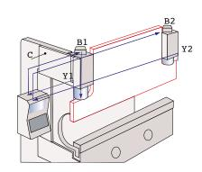
The upper beam is guided by 4 pairs of bearings that slide, along the machine's sides, on tracks of hardened and rectified steel. The alignment and centering of the beams is guaranteed by the great distance between the upper and lower bearings (E). Both the optical scales (Y1 and Y2) are mounted on two plates (C) shaped as the side's throat and fixed to the lower beam. Moreover, the optical scales are connected to the CNC, allowing to control the oil flow through the servo-valves (B1 and B2).
