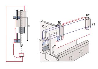
The upper beam is guided by 4 pairs of bearings that slide, along the machine's sides, on tracks of hardened and rectified steel. The alignment and centering of the beams is guaranteed by the great distance between the upper and lower bearings (E). Both the optical scales (Y1 and Y2) are mounted on two plates (C) shaped as the side's throat and fixed to the lower beam. Moreover, the optical scales are connected to the CNC, allowing to control the oil flow through the servo-valves (B1 and B2).
